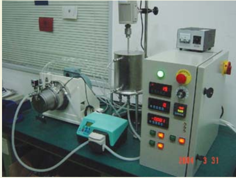
0.3 L grinding and dispersion equipment prototype (2004, 03)
