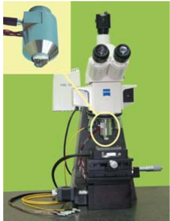
Microscope Objective Type AFM (with mini-size AFM probe module/build-in scanner)
