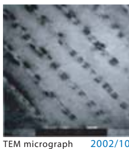
Stacked 10 layers InAs/InGaAs quantum dot laser structure on GaAs substrate
